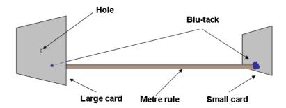
Point the end with the hole towards the Sun. Adjust the alignment of the metre rule carefully until you can see a small image of the sun projected onto the lower card. The Sun's disk might be difficult to see due to sunlight. The larger card on the front of the rule should provide a little shade but you may need to get your friends to stand around the smaller card to help create some more shade.
